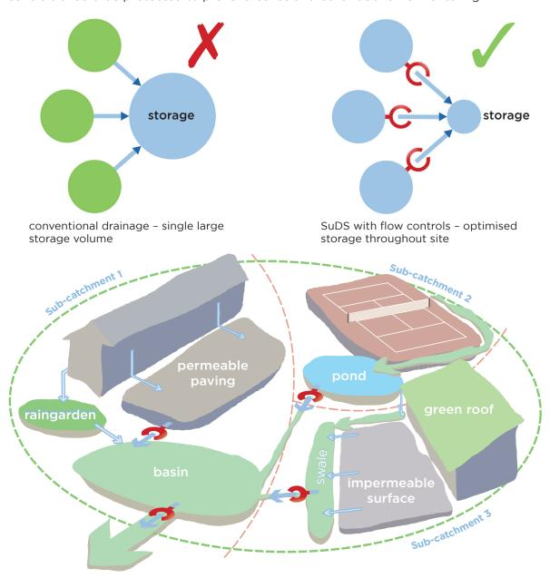
With their low cost and shallow construction, Controflow® chambers are ideally suited to control flows from each sub-catchment as well as from whole sites, while realising a key aim of SuDS to keep water management on or near the surface.
