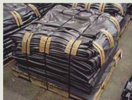
Prefabricated liner ready for dispatch
